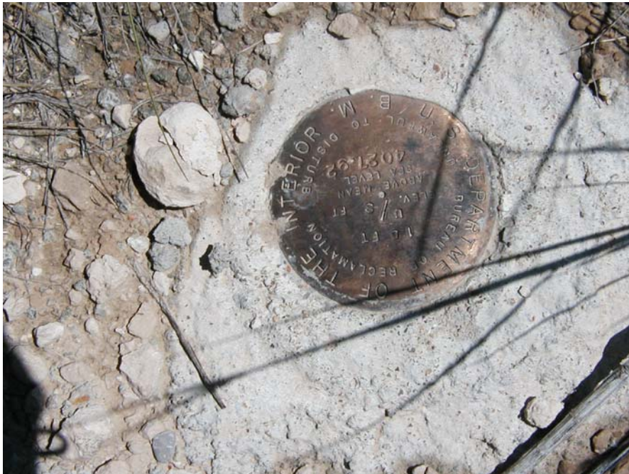
Figure 3 - BOR cap, left abutment, u/s 15-feet, elevation 4027.92.
